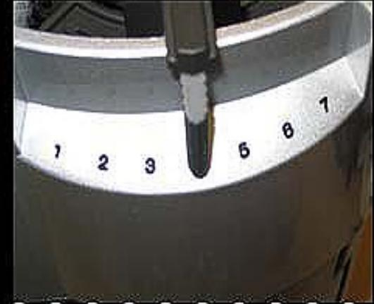
**Step 10:** Now the grinder setting arm needs to be placed back onto the outer-ring (little holes around it). Drop it down and snap in place at the # 4 grinder setting.
