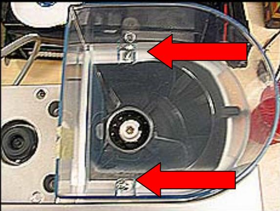
**Step 11:** Now place the bean container back on the unit and tighten down with the 2 Phillip Screws that were removed at the start.
