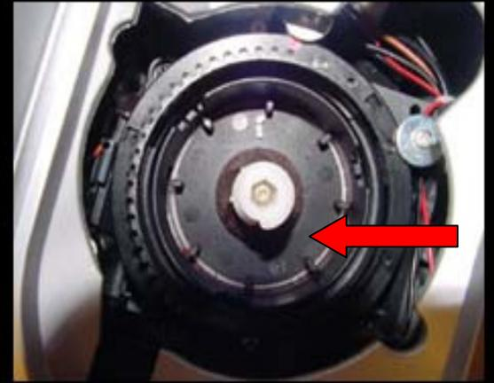
**Step 6:** This area should be vacuumed so that all coffee beans and grinds are removed.
