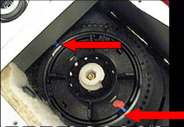
**Step 8:** Turn the outer ring counter clockwise until the blue stripe on the outer ring is 180 degrees opposite from the one on the inner ring.
