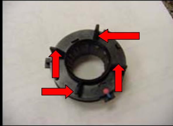
**Step 5:** This is the inner ring [burr] shown above that you will be lifting up on. The arrows are pointing to the four tabs to lift up on.
