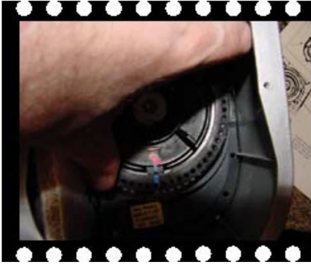
**Step 4:** Turn the outer ring counterclockwise until the two blue lines are aligned and lift the inner ring from the grinder assembly.
