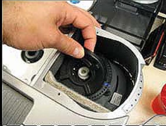
**Step 9:** Now place the black rubber gasket back down onto the inner part (burr).
