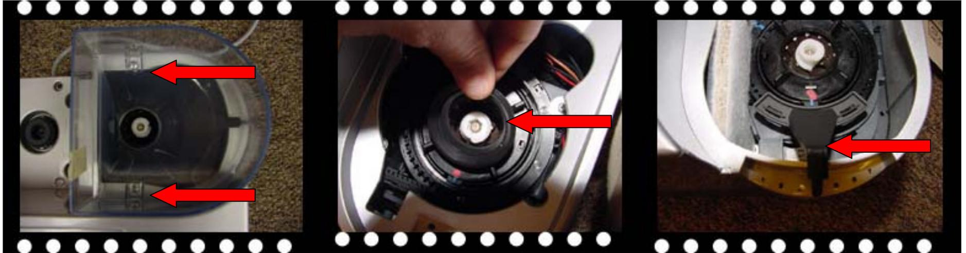
**Step 1:** Make sure the machine is turned off and unplugged. Remove all beans from the bean container. Vacuum out all the beans that cannot be scooped out. Remove 2 philips head screws from bean container. Remove the bean container from machine by pulling straight up.
